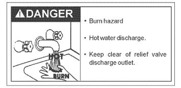
When checking the temperature-pressure relief valve operation, make sure that (1) no one is in front of or around the outlet of the temperature-pressure relief valve discharge line, and (2) that the water discharge will not cause any property damage, as the water may be extremely hot, see Figure 24.
